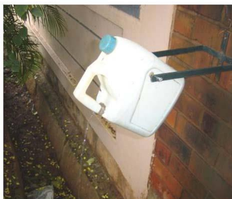
Water "tap" for washing hands using 0.1 litre per hand wash
